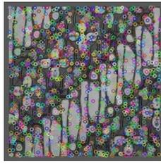
Figure 3. SIFT keypoint in Batik Parang.
