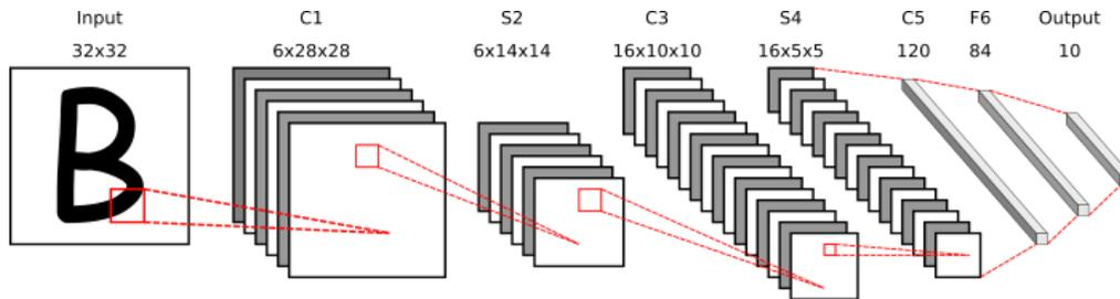
Figure 4. LeNet5 convolutional network
